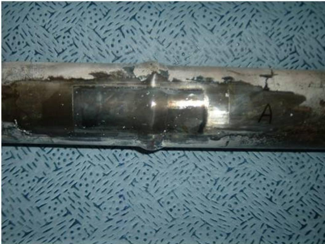
The test subject was T23 boiler tube applied to a power plant, and the attachment of V-block system was applied. Test purpose was to evaluate properties and residual stress of weldment before and after heat treatment. The actual evaluation result confirmed that the residual stress was stabilized and tensile properties were maintained by the conditions of heat treatment..
