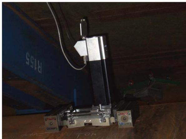
**Curvature magnet system - Long Dovetail Slider**
