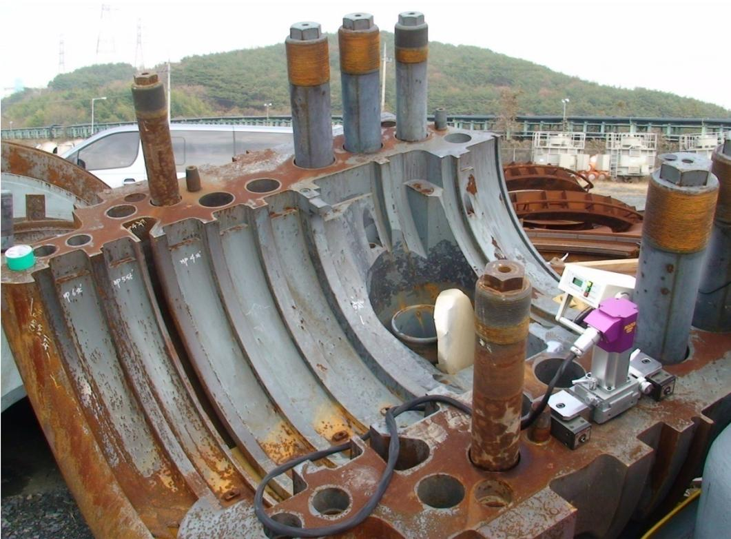
The test subject was turbine rotor case, and flat magnet system was applied, considering the shape. Purpose of the test was the evaluation of abrasion degree and life span, and the required properties evaluation was carried out.
