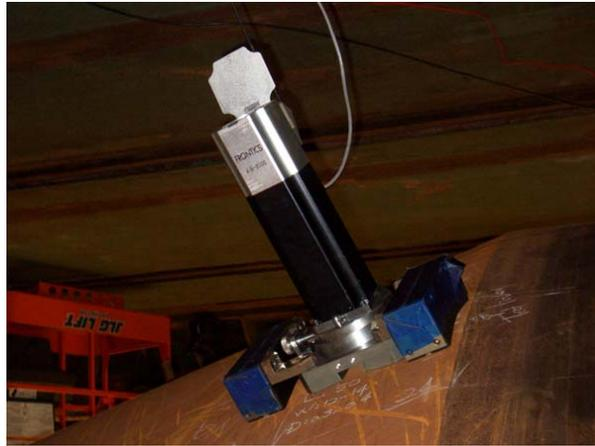
**Curvature magnet system - Dovetail Slider**
