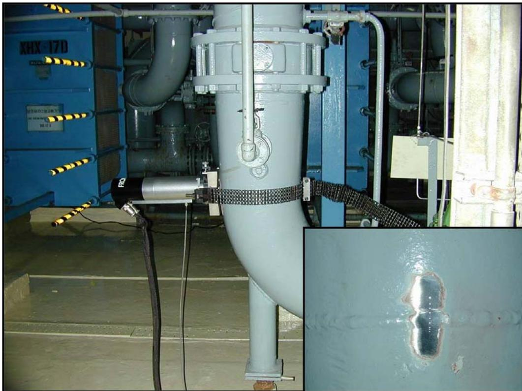
The test subject was cooling water line of a nuclear power plant, and chain system was applied, considering the shape. Test location was the weldment of elbow and pipe, and we have evaluated the properties change during last 20 year use.
