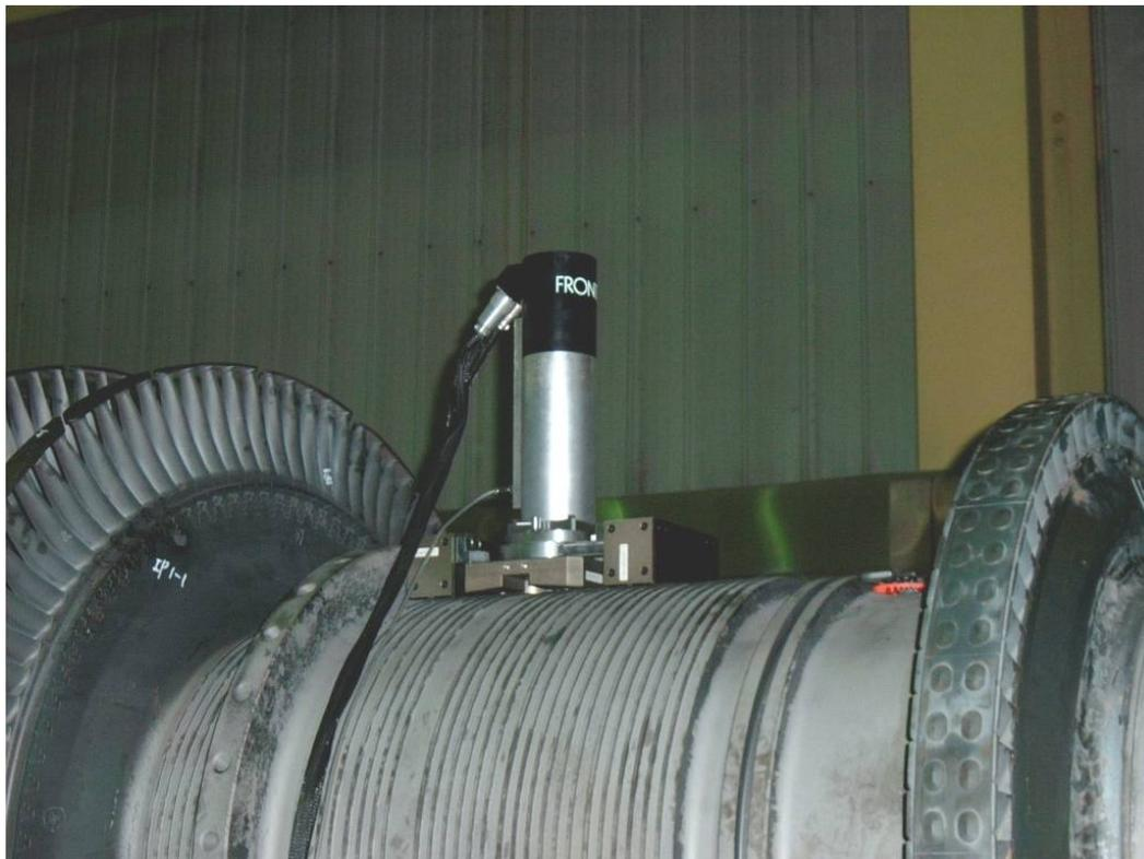
The test subject was a turbine rotor used for 22 years, and the test was conducted by applying curvature magnet system, as the shape was circular. Unusual point was that the test spot located in a narrow region 15 – 30 mm inside uneven section.
