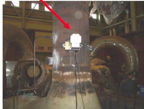
The test subjects were ICV, IP Rotor and Turbine casing of a thermal power plant. We have tested them applying lightweight chain system and flat magnet system, as sizes of the test regions were different.
