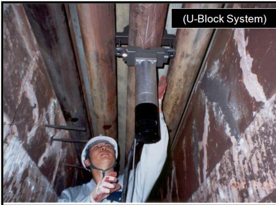
The test subject was heater tube of an oil refinery plant. U-block and V-block were applied depending on the size of the subject. Purpose of the test was the evaluation of aging of the material on use and PQ test of the new material.
