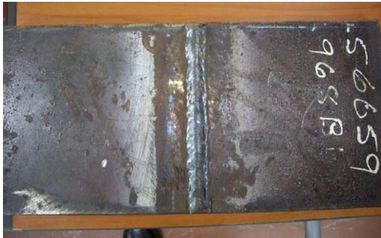
The test subject was specimen welded with API X65 plate, and we applied RS-MPS that was expansion of MPS, considering the shape. Purpose of the test was to evaluate properties and residual stress of weldment.
