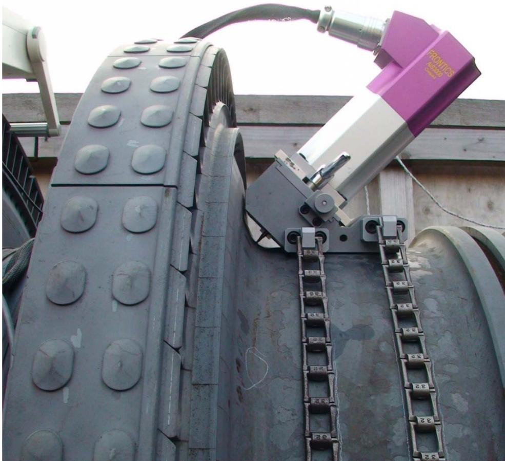
The test subject was HP rotor, and the location of the test was groove section. We made the special attachment system that was applied to the test, considering the shape. Purpose of the test was to estimate finally the lifetime by evaluating the physical properties of the subjected section.
