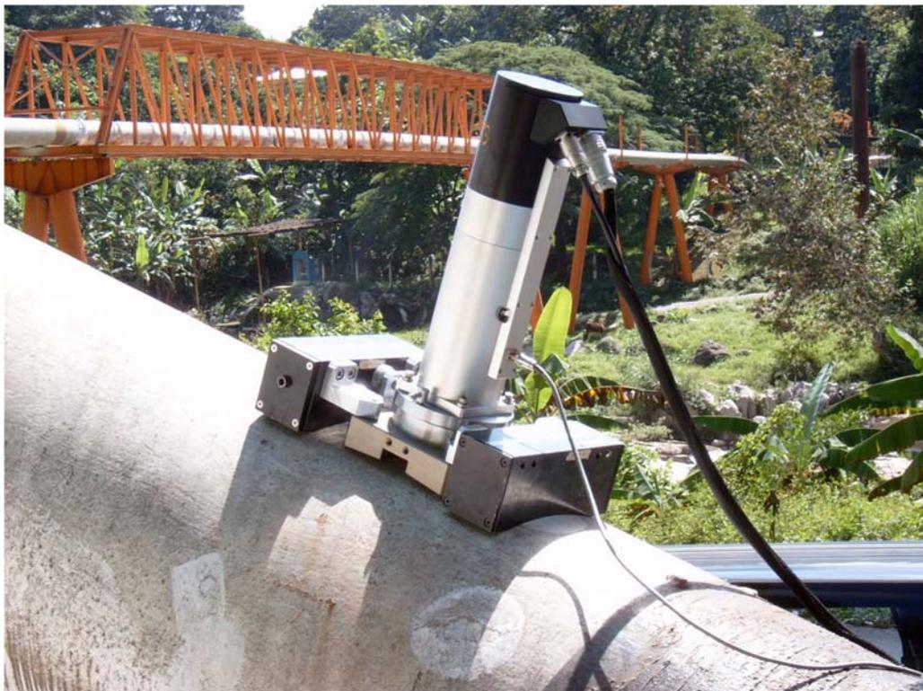
The test subject was natural gas pipeline that had been installed and operated in Mexico. Considering the shape of the subject, curvature magnet system was applied. The target subject was the exposed pipelines and the underground ones, and aging of the materials was evaluated as well. (Refer to Oil and Gas Journal Vol. 101(2003) pp66-71)
