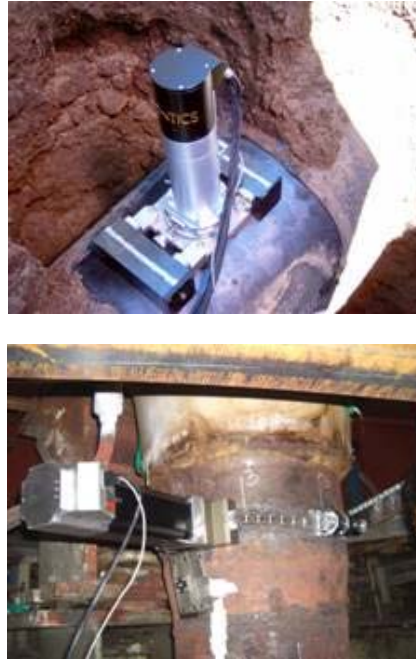
Fig. 7 Examples of indentation technique application for in-service inspection
