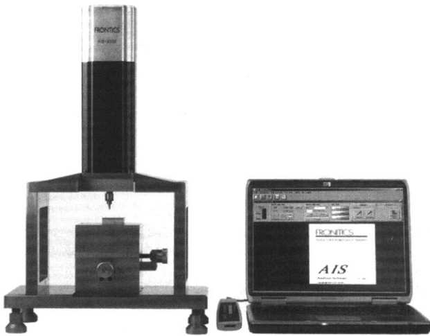
Fig. 1. AIS3000 of Frontics, Inc. used for residual stress measurement on local region.
